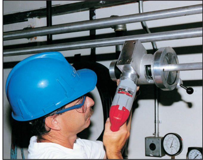
Solution Profile: The portable Model 303, performing tube squaring in a low clearance situation. This Model 303 was specially configured to operate within a customer's custom size range.
