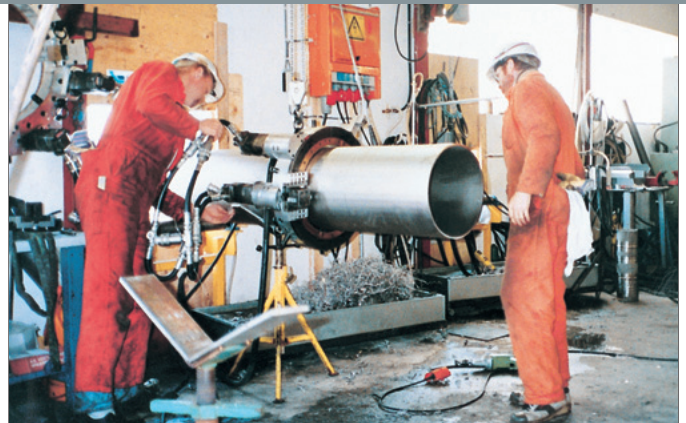
Solution Profile: While most often used in a portable role, clamshells are extremely effective in fab shops where high volume, precise severs, bevels and end preps are needed. The above Clamshell is shown performing a sever/bevel on titanium.
