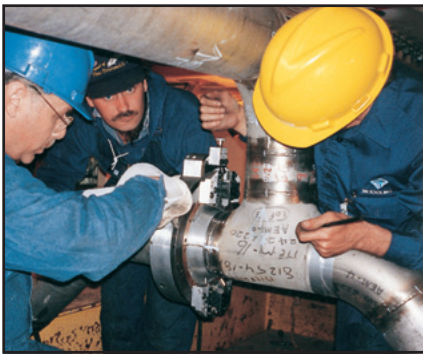
Solution Profile: Accurate, reliable machining in tight spaces is what the clamshell lathe does best, reducing the downtime and labor required for plant maintenance operations, while ensuring quality welds.
