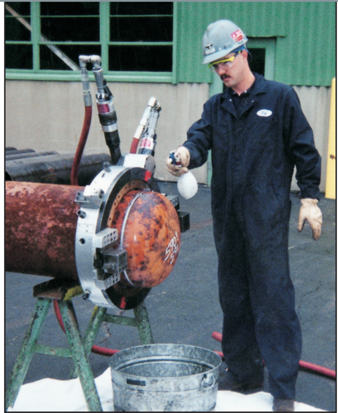
Solution Profile: A Model 616SB lathe with dual pneumatic motors performing a sever/bevel operation to cut off the end of a pressure vessel.
