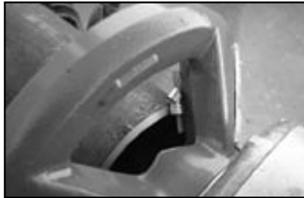
The 4X4™ Beveler's cutting head offers a full safety cage, but still provides excellent visibility of the cut with the "chip" indicating the optimal feed rate.
