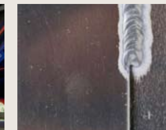
The MIX TIG function combines the good qualities of direct and alternating current. It makes joining aluminium materials easy and decreases the number of deformations.
